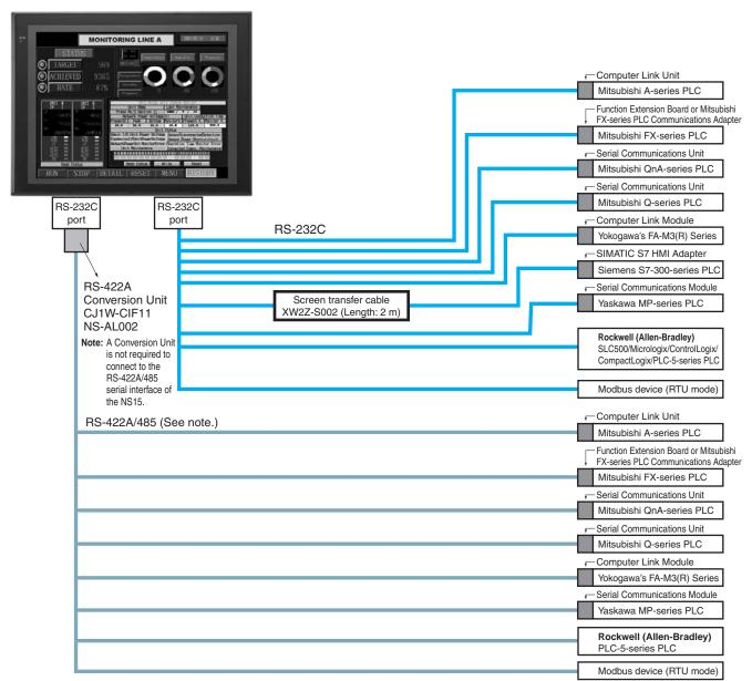
Note: Whether an RS-422A or RS-485 connection is supported depends on the device that you are connecting to.
